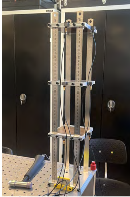
Figure 3.4: three-story frame structure in the laboratory.
